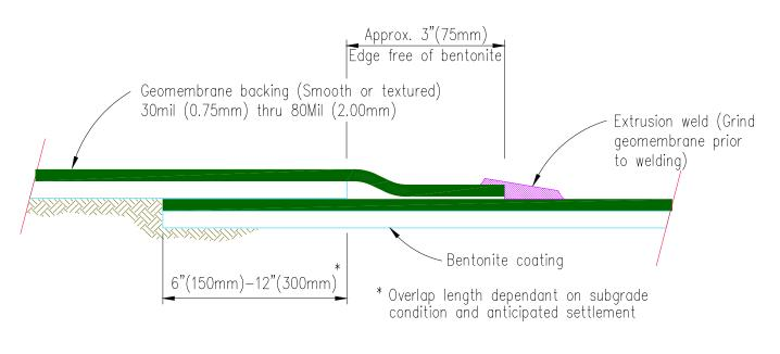
Gundseal Extrusion Welded Seam
